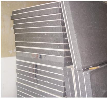
3 Composite panels from plaster board (white) and insulating boards of Neopor (silver-grey)
